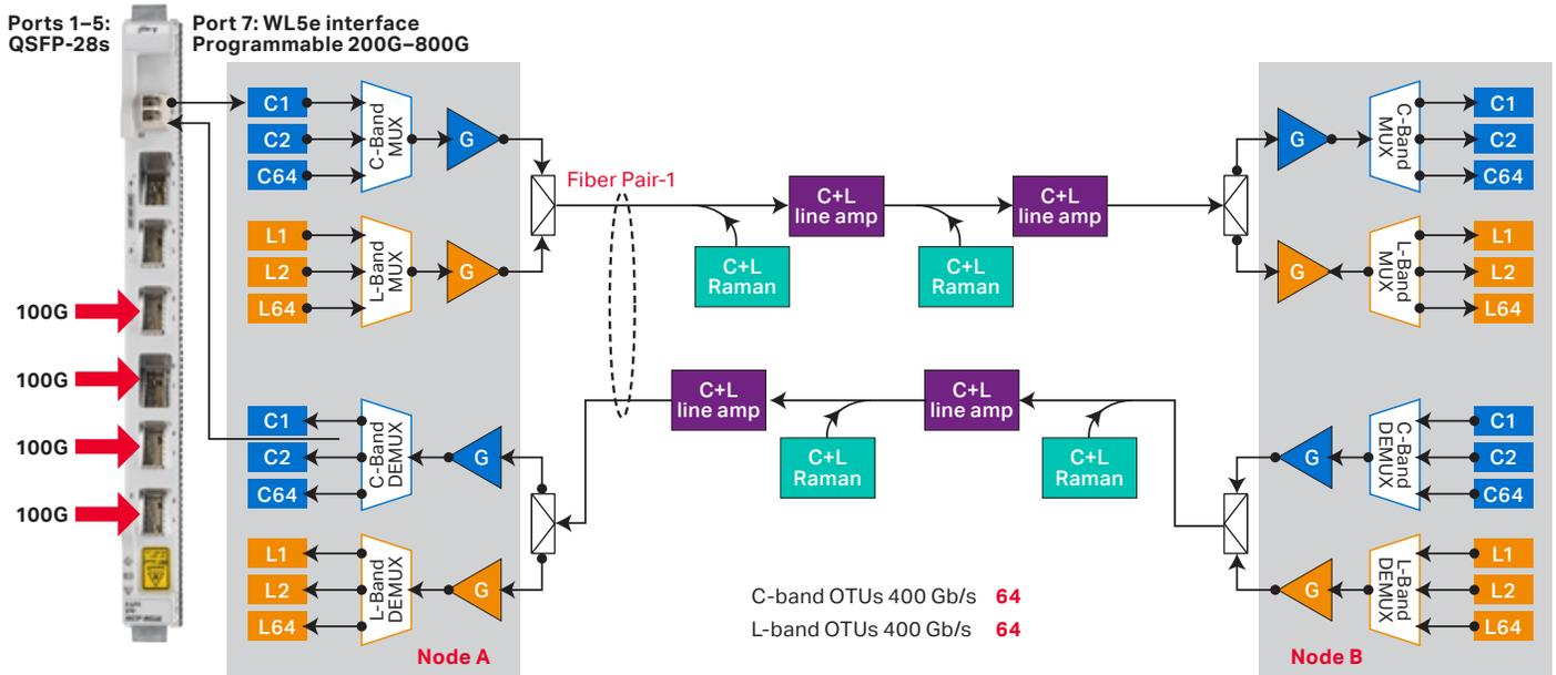
Figure 5(ii). Managed spectrum/wavelength service based on Ciena’s integrated C&L-band architecture
